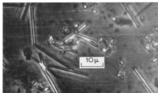
Figure 1 Polycarbonate. Simple needle crystals in film prepared from xylene slurry. Phase contrast.
